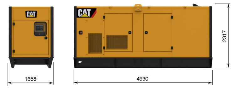
Approximate weight of enclosure package: 5280 kg (11,640 lb). Exact weight is dependent on options. Enclosure weight includes: sound attenuated enclosure, exhaust system, base and generator set. Generator set enclosure also available in white. (Caterpillar yellow is standard colour)
